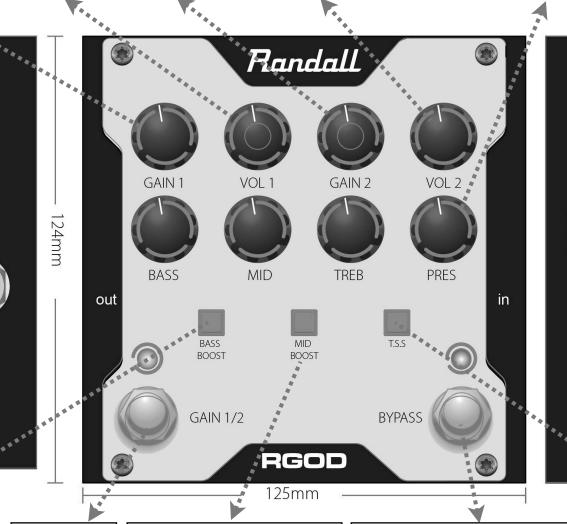
Connect included PPS1 external power supply unit here. Positive or negative center power supplies will work with a minimum of 9volts.
