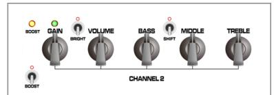
GAIN: Overall gain control for clean channel. Use this control along with the volume for ranges from crystal clean to slight break up.
