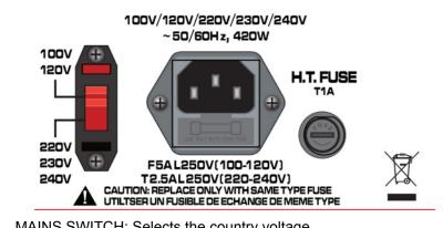
MAINS SWITCH: Selects the country voltage. For 100-120VAC selections, change IEC fuse to T5A/250V fuse. For 220-240VAC selections, change IEC fuse to T2.5A/250V fuse. The H.T. Fuse remains unchanged.
