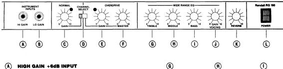
This input accommodates most musical instruments. The gain characteristic of this input is 6dB higher than the low gain input.
