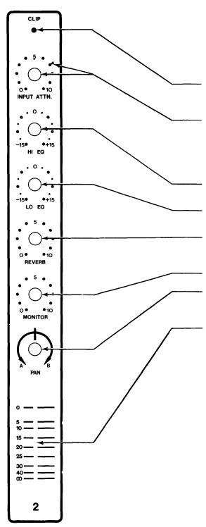
LED Light at the top of each channel indicates clipping in the pre amp. The light actually will come on 5 dB before clipping.
